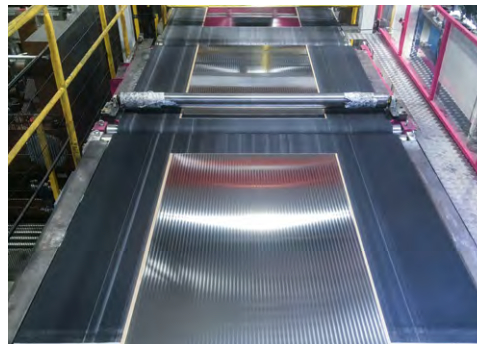
Cut-to-length line for up to 2,150 mm wide sheets
